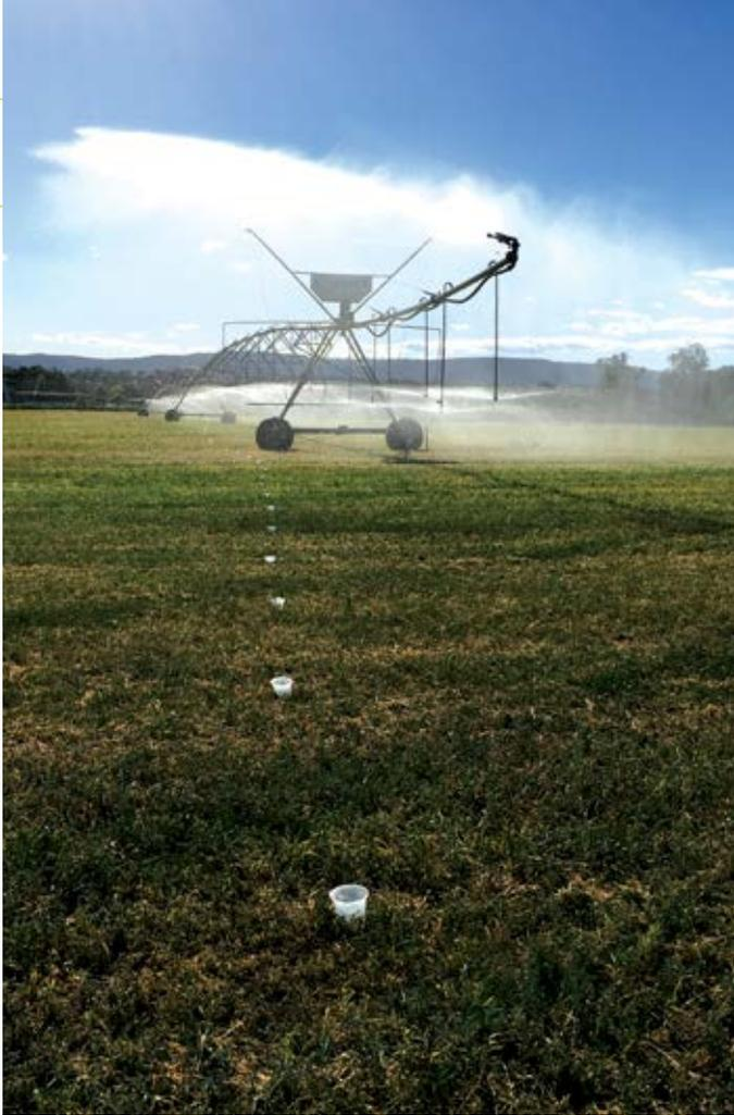
Randomly selecting up to 20 sprinklers and checking flow rate measurement using is a recommended way for judging the condition of a sprinkler package. *Photo: Peter Smith*
